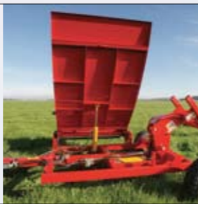
Pivoting steel floor for effective and efficient feed out
