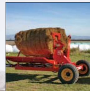
Bale held in position ready for string removal
