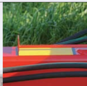
Position indicator of rear loading mechanism
