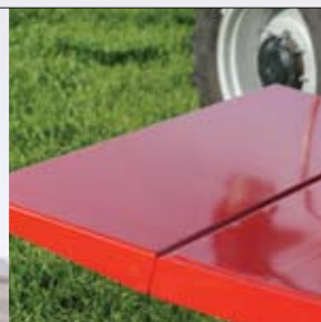
Extendable floor to accommodate large bales
